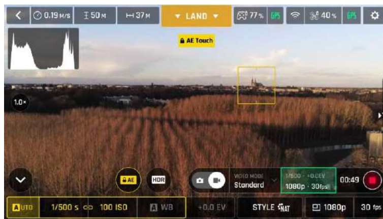
Exposure is locked on a building on the horizon (Android): shutter speed is set at 1/500 s
