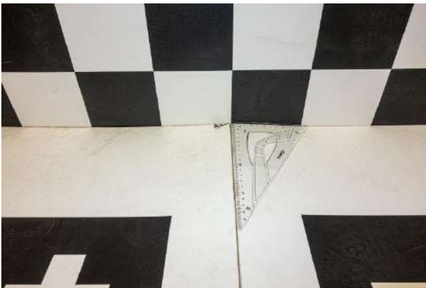
Finding a line perpendicular to the wall
